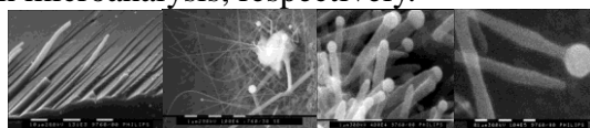
Fig. 1. Micrographs FNSG: a) Ti- OOMS at 850°C; b) Zr - OOMS at 1350°C ; c) Hf - OOMS at 1350°C ; d) Ta- OOMS at 1350°C .
